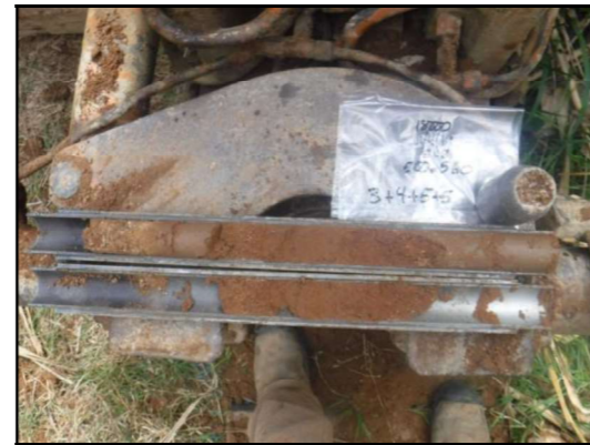
Foto 20: Sondeig Sv-8, SPT a 5,0 metres.
