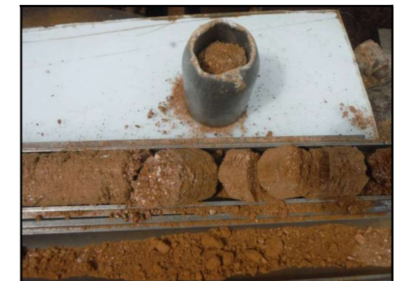
Foto 4: Sondeig Sv-1, SPT a 7,0 metres.
