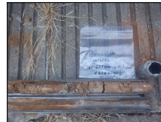
Foto 14: Sondeig Ss-5, SPT a 1,0 metre.
