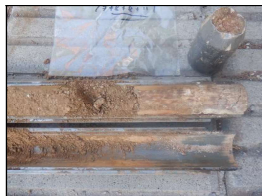
Foto 11: Sondeig Ss-4, SPT a 1,0 metre.
