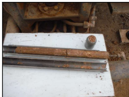
Foto 11: Sondeig Sv-5, SPT a 7,0 metres.
