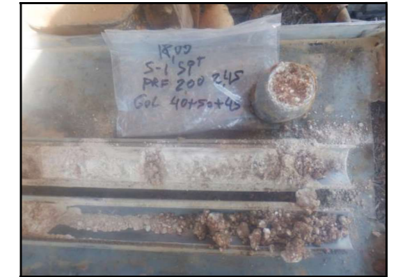
Foto 2: Sondeig Ss-1, SPT a 2,0 metres.
