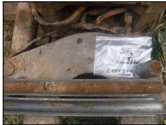
Foto 19: Sondeig Sv-8, SPT a 2,0 metres.
